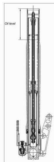
First see manual. The modern front fork of cartridge type is very sensitive to oil level changes, because of the small air volume.
